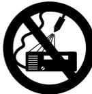
Never direct the high-pressure jet or water hose against the machine itself or against other electrical appliances and equipment – **danger of short-circuiting!**
